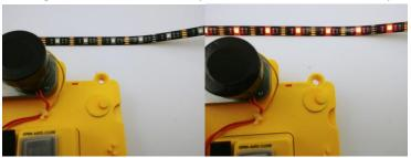
e. Set blast gate mode to "OPEN". Blast gate slide shall move to open position. Red LEDs shall be off when slide stop at the fully open position.
