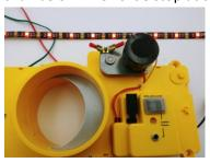
f. Position a Source Tab at the top left corner around 0.75" from the top and 0.25" from the left edge. Adjust the position until the green LEDs are on. Mark position, remove the backing of the double sided tape and secure Source Tab in position.
