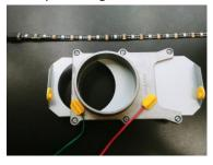
c. Fully close the gate. Red LEDs are on and Green LEDs are off.
