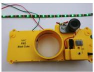
b. Move the mode switch to "CLOSE". Slide will start moving to right. Green LEDs will remain on and Red LEDs will be on too.
