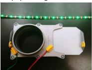
b. Half open the gate. Both Green and Red LEDs are off.
