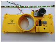
c. Green LEDs will be off when the slide arrives at the fully closed position.
