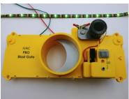
Red LEDs will be off when slide arrives the fully open position.
