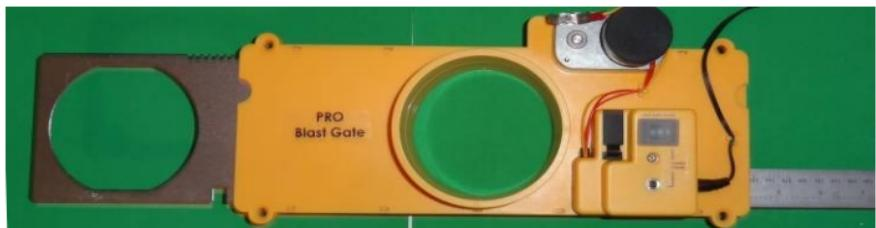
The Slide can now be cleaned with an appropriate solvent. (WD40 or Varsol). Solvent should **NOT** be used on the ABS plastic part of the Blast Gate. Dust should be blown off using compressed air. After cleaning you can replace the slide from the left until it is even with the left side. Reconnect the power and test using the mode switch.
